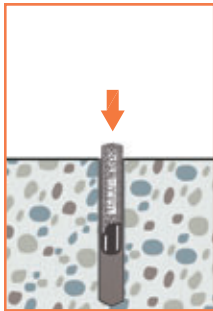
Insert KLP capsule into drilled hole
